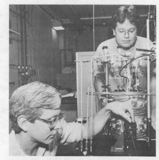
WHILE GEORGE WILKERSON (8353, right) looks on, Joe Durant (8353) aligns the fiber-optic output coupler of a laser photolysis/laser-induced fluorescence apparatus in CRF's Chemical Kinetics Lab. This and other research tools help scientists learn more about elementary gas phase reactions important for thorough analysis of the combustion process.
